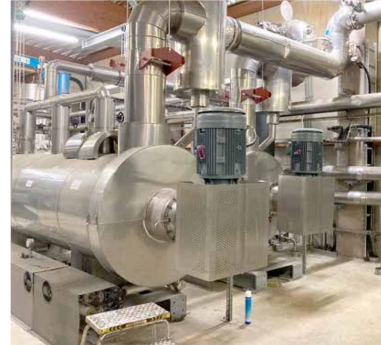
The thin-film dryers, above the droplet separator and to the right the insulated condensers. © GIG Karasek
