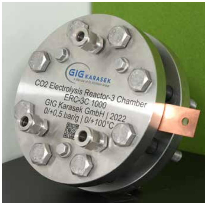
Patented ECO2CELL electrolysis cell © GIG Karasek
