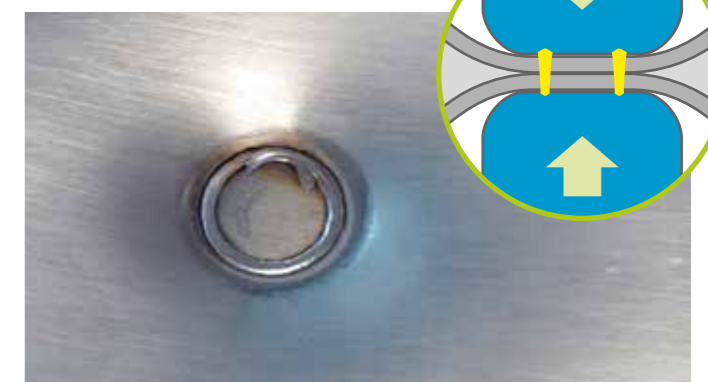
LASER Luxe Lamella - Ring-shaped weld seam with laser welding © GIG Karasek
