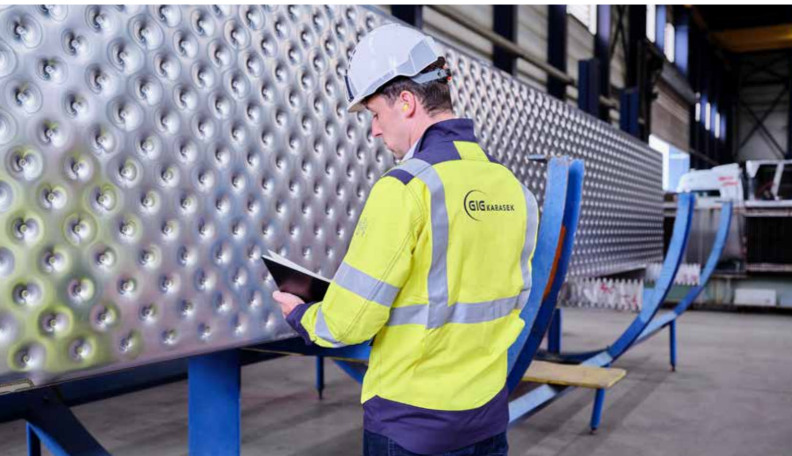
Lamella bundle manufactured at our production facility © GIG Karasek
