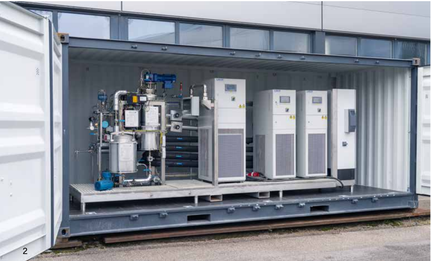
Short-path evaporator MINIPLANT for the distillative purification and recovery of valuable materials © GIG Karasek
